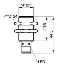
Inductive Sensors BES 516-355-G-E5-Y-S 4 M18x1 x 44.5 normally-open Sn=8mm shielded
